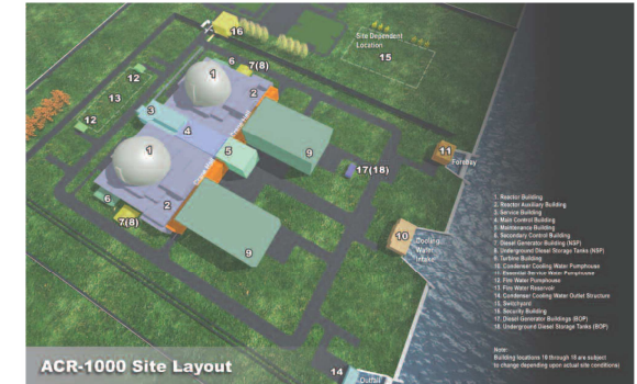
Figure 2-1 Two-Unit Plant Layout of Major Structures
