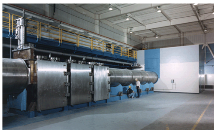
The separator demonstration facility at Lawrence Livermore's laser isotope separation (LIS) plant plant tested full-scale equipment. One of three separator units shown for enriching uranium was operational for demonstrations. Also visible are beam tubes for transporting precisely tuned laser light to the separator units.
