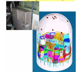
Hydrogen Removal System
