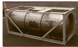
Uranyl nitrate, transported in LR 65 tank-container (size : ISO 20 ft) (Type IP-2 package)
