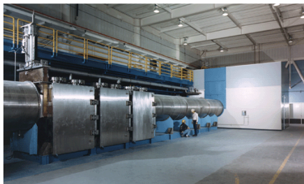
The separator demonstration facility at Lawrence Livermore's laser isotope separation (LIS) pilot plant tested full-scale equipment. One of three separator units shown for enriching uranium was operational for demonstrations. Also visible are beam tubes for transporting precisely tuned laser light to the separator units.
