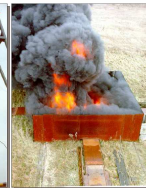
9 meter high drop test, and 30 minutes long fire
