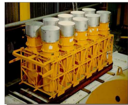
PuO 2 powder, transported in FS 47 casks (Type B(U)F packages)
