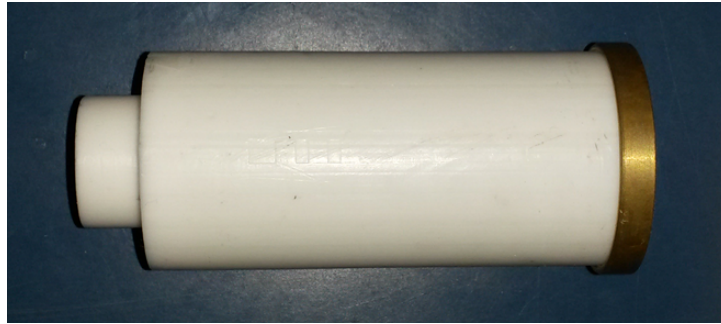
Figure 5.10: Teflon tube with a copper ring on it used to tune the Sodium coil.
