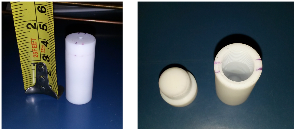
Figure 8.8: Cylindrical water phantom for x gradient efficiency measurement. Left: Closed sample holder. Right: Opened sample holder with the water in it.
