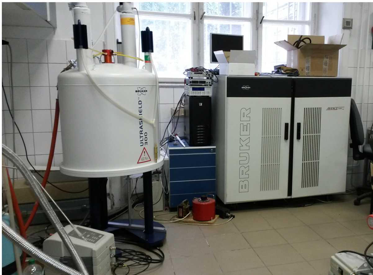
Figure 3.1: The used NMR spectrometer (right) and the shielded superconducting magnet (left).
