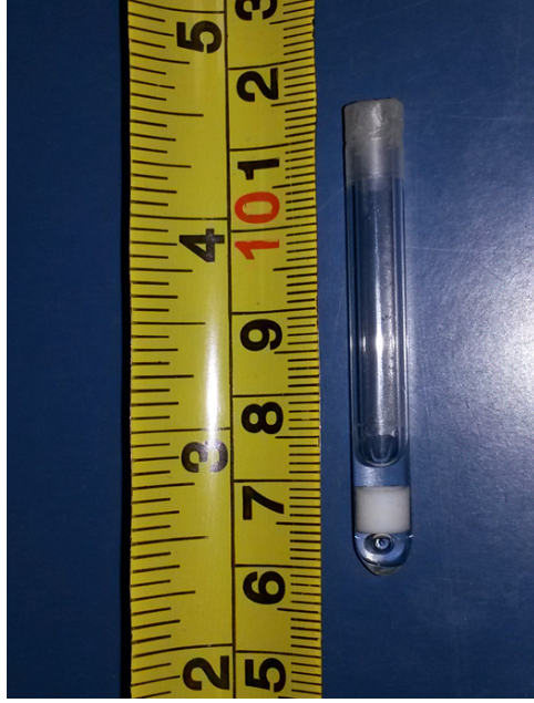
Figure 8.6: Quartz tube with two water parts separated by a teflon plug; a phantom used for z gradient efficiency measurement.
