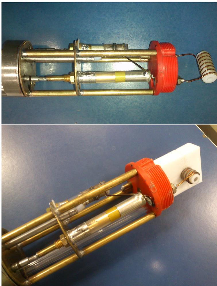
Figure 3.1: The constructed NMR probe for broadband, low frequency measurements
