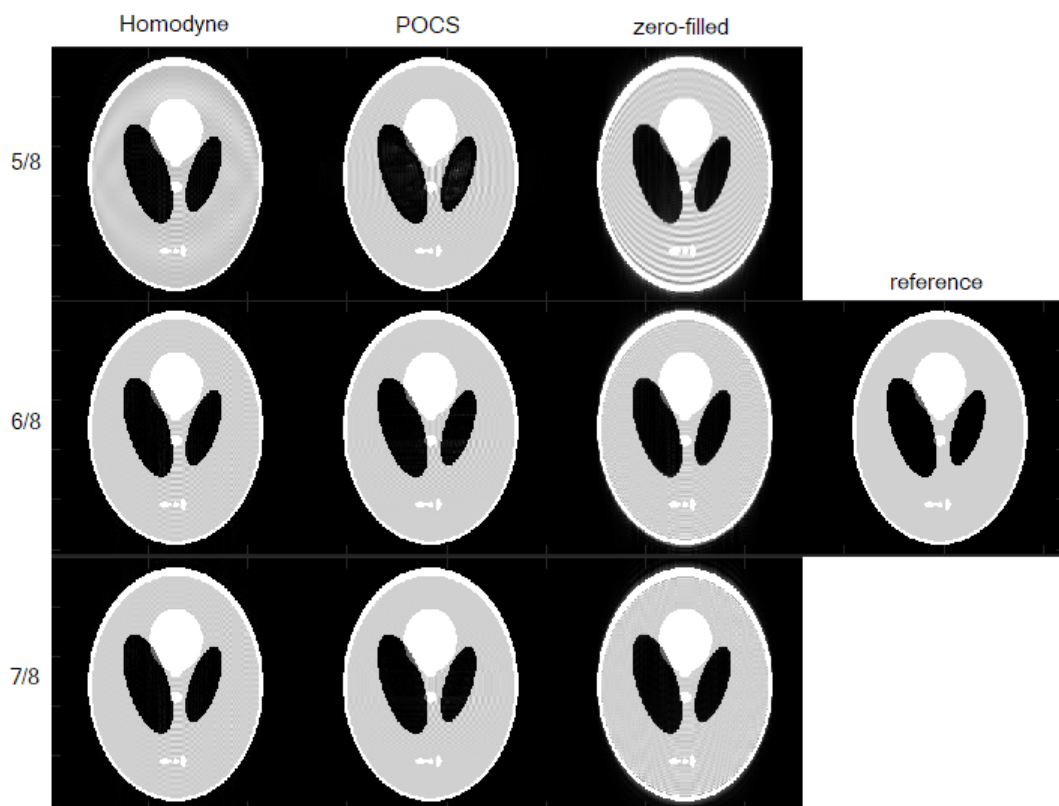
Figure 27: Shepp Logan phantom reconstructed with partial Fourier factors 5/8 , 6/8 and 7/8 , with a full data set as reference.
