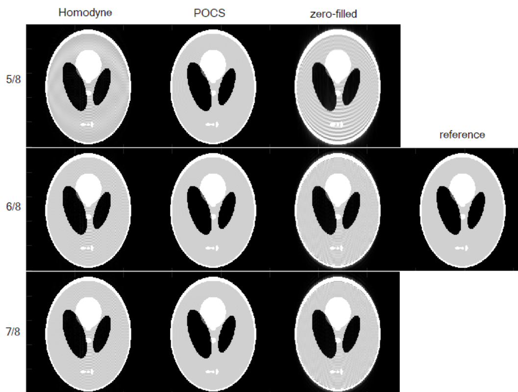
Figure 19: Shepp Logan phantom reconstructed with partial Fourier factors 5/8 , 6/8 and 7/8 , with a full data set as reference.
