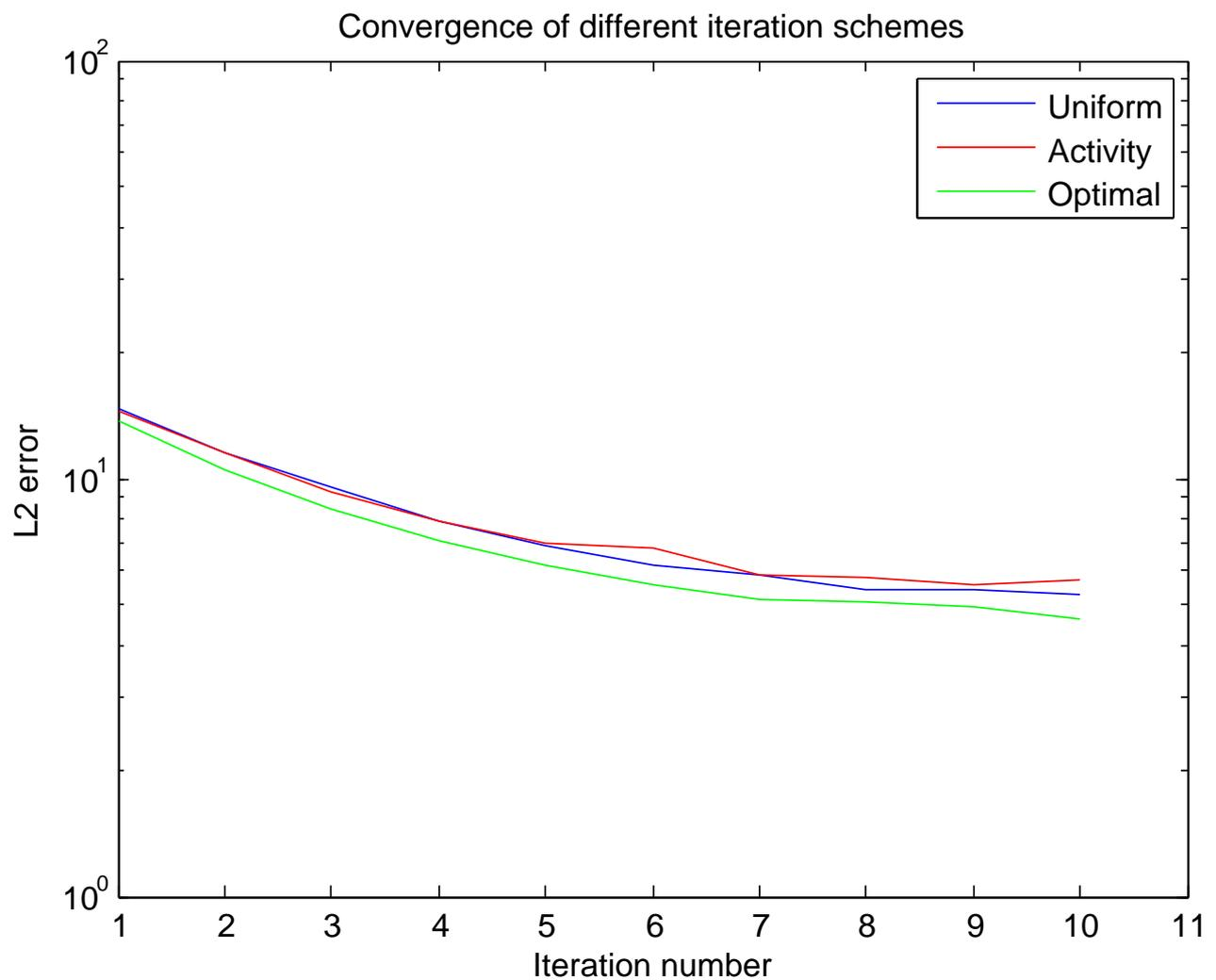
Figure 8.1: The log-linear plot shows total squared error of reconstructed activity values as a function of iteration number. It can be seen that choosing between uniform and activity weighted sampling in the back projection step has little to no effect, while the optimal sampling performs slightly better than the rest. System matrix:  $[0.3, 0.1; 0.4, 0.8]$ , activity concentrations:  $[1, 9]$
