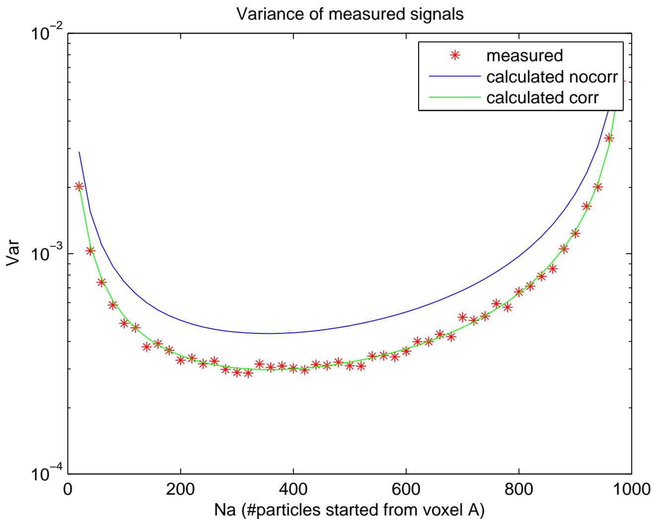
Figure 6.2: Log-linear plot of variance results. It is clear that simulated and calculated results accounting for correlations are in agreement. Neglecting correlations causes a slight deviation from simulated values.
