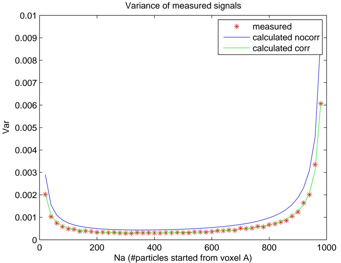
Figure 6.1: Linear plot of variance results. It is clear that simulated and calculated results accounting for correlations are in agreement. Neglecting correlations causes a slight deviation from simulated values.
