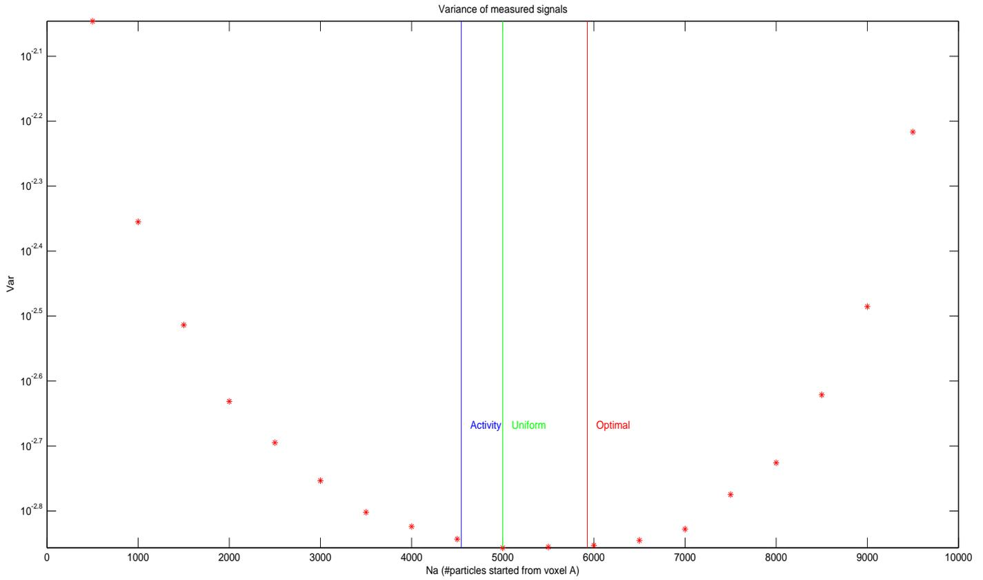
Figure 6.3: Total variance of the ratio of measured and simulated LOR counts. Red markers show simulation results, while vertical lines show what portion of all virtual particles the different samplings appoint to voxel A. System matrix:  $[0.1, 0.04; 0.4, 0.05]$ , voxel activities:  $[1, 12]$ .
