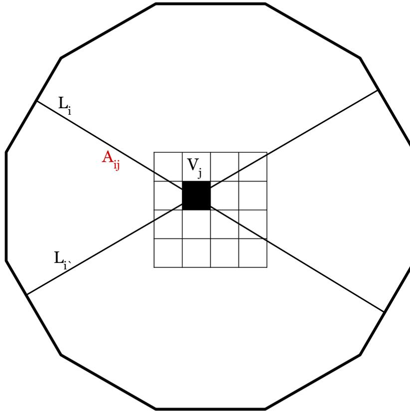
Figure 1.1: The real system is discretized into voxels (square grid in the centre), while the imaging device consists of detector panels (sides of the regular polygon). Each detector pair constitutes a LOR; and coincidence detection in the two detectors translates to a particle detection in their LOR. Two LORs are shown:  $L_i$  and  $L_i'$ . The system matrix element  $A_{ij}$  is the probability that a photon pair emitted from voxel  $V_j$  gets picked up by LOR  $L_i$
