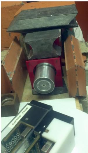
(a) Experiment set-up with  $Cs - 137$  point source using a lead collimator.
