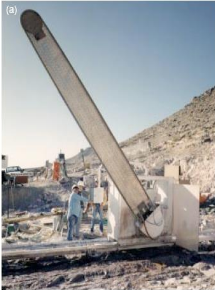
Figure 2. (a) Rock was cut out of Yucca Mountain in Nevada and (b) tested to determine hydrologic and geochemical characteristics.
