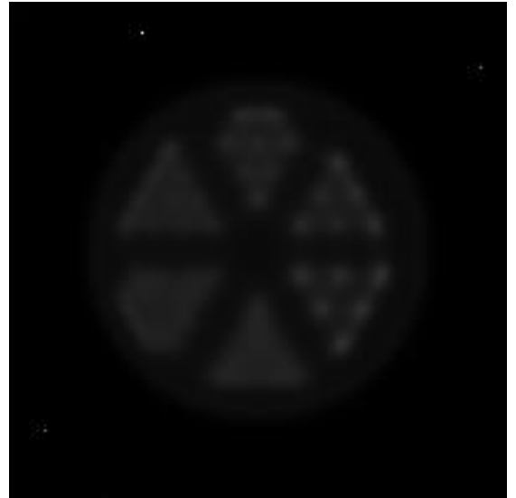
Figure 51: Resulted salt and pepper - like noise accumulation in the reconstruction. The subsequent ML-EM iteration step gave only a pattern similar to a Dirac-delta and the reconstruction is broken
