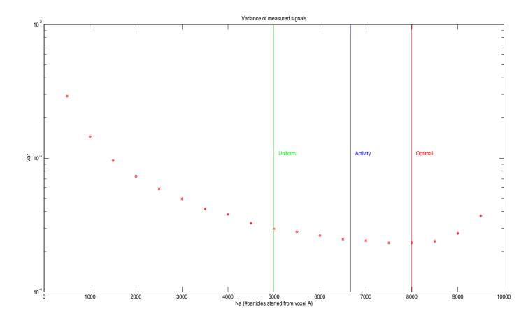
Figure 6.4: Total variance of the ratio of measured and simulated LOR counts. Red markers show simulation results, while vertical lines show what portion of all virtual particles the different samplings appoint to voxel A. System matrix: [0.1, 0.45; 0.15, 0.5], voxel activities: [1, 12].
