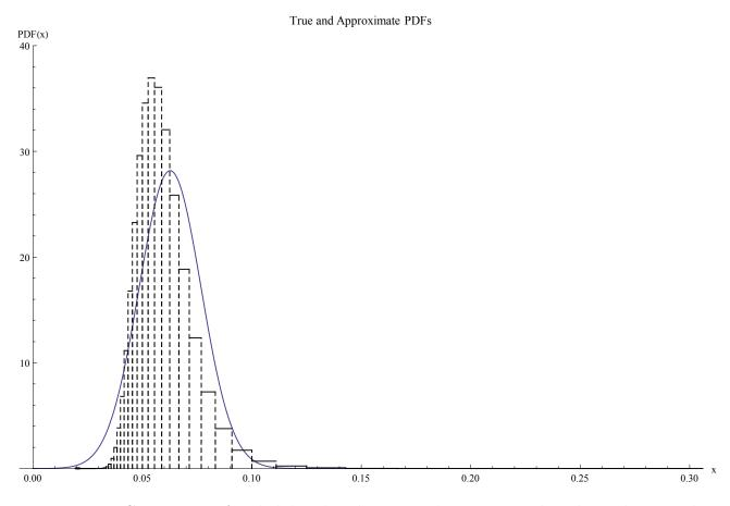
Figure 2.1: Comparison of probability distributions. The continuous line shows the normal approximation, while the dotted lines show a normalized histogram of the true distribution of values. In this case n = 50 and  $p = \frac{1}{3}$
