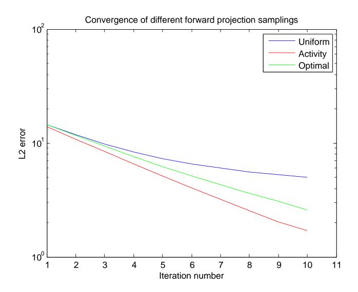
Figure 8.2: The log-linear plot shows total squared error of reconstructed activity values as a function of iteration number. It can be seen that uniform is significantly worse than either of the others. Furthermore activity weighted sampling performs better than the theoretically derived optimal sampling. System matrix: [0.3, 0.1; 0.4, 0.8], activity concentrations: [1, 9]
