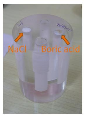
(a) Used phantom: polyethylene cylindric sample holder (5 cm diameter, 10 cm height) filled with boric acid and table salt.
