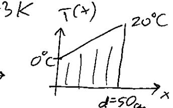
$$\text{Így a fel grad} T-t: \quad \text{grad} T = \begin{bmatrix} \frac{\partial T}{\partial x} \\ \frac{\partial T}{\partial y} \\ \frac{\partial T}{\partial z} \end{bmatrix} = \begin{bmatrix} \frac{T_2 - T_1}{d} \\ 0 \\ 0 \end{bmatrix} = \begin{bmatrix} 40 \\ 0 \\ 0 \end{bmatrix} \text{K/m}$$
