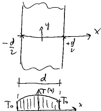
$$x = \frac{d}{2}: T_0 = -\frac{1}{2} \frac{\dot{e}}{n} \left(\frac{d}{2}\right)^2 + A \frac{d}{2} + B$$
