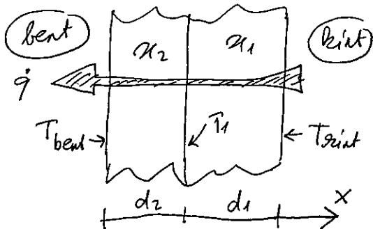
$$\gamma_1 = \frac{d_1}{\lambda_1} = \frac{0,25\text{ m}}{0,77 \frac{\text{W}}{\text{mK}}} = 0,3247 \frac{\text{m}^2\text{K}}{\text{W}}$$
