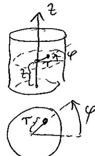
$$\frac{\partial T}{\partial t} = a \cdot \left[ \frac{\partial^2 T}{\partial r^2} + \frac{1}{r} \frac{\partial T}{\partial r} + \frac{1}{r^2} \frac{\partial^2 T}{\partial \varphi^2} + \frac{\partial^2 T}{\partial z^2} \right] + \frac{1}{S \cdot c_p} \cdot \dot{e}$$
