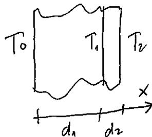
$$\gamma_1 = \frac{d_1}{\kappa_1} = \frac{0,3m}{0,5 \frac{W}{mK}} = 0,6 \frac{m^2K}{W}; \quad \gamma_2 = \frac{d_2}{\kappa_2} = \frac{0,03m}{0,15 \frac{W}{mK}} = 0,2 \frac{m^2K}{W}$$
