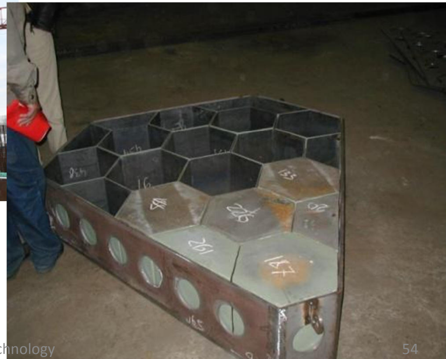
Sacrificial material of the core catcher
